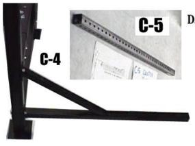
D. REAR CENTER TIE BAR (C5) SLIDES INTO REAR SUPPORT (C4) AND AFTER ADJUSTED IS BOLTED INTO PLACE USING 1 BOLT, WASHER, LOCK WASHER, NUT--PER SIDE
