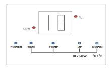
6) To find the ambient room temperature, hold down the TEMP + TIME and then let go. The ambient temperature will be displayed. To calibrate temperature setting, hold down the TEMP button for (5) seconds to switch to thermostat calibration status. The LED display
