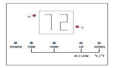
Press TEMP to switch to temperature status, then press HI/LOW/UP button once within 5 seconds to scroll up
