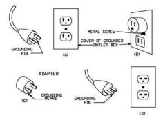
available for connecting three-blade grounding-type plugs to two-slot receptacles. The grounding lug extending from the adapter must be connected to a permanent ground such as a properly grounded outlet box. The adapter should not be used if a three-slot grounded receptacle is available.
