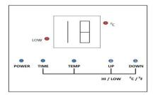
6) To find the ambient room temperature, hold down the TEMP + TIME and then let go. The ambient temperature will be displayed. To calibrate temperature setting, hold down the TEMP button for (5) seconds to switch to thermostat calibration status. The LED display
